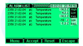
The **Alarm List** is displayed with most recent alarms at the top with eight messages per page. The alarm list holds the last 100 alarm messages generated for the system. Each message includes the time and date of occurrence, the system reference number and the reason for the alarm.
