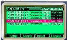
Alarms Limits and guard time delays for each temperature zone are easily adjusted using the 'Setup' menu
