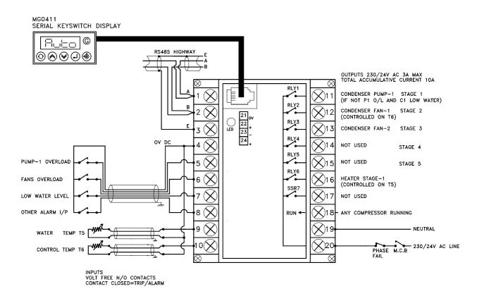
COOLING TOWER RUNS IF RUN SIGNAL FROM ANY HT COMPRESSOR.
