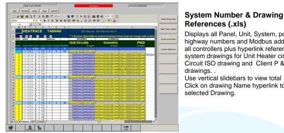
Displays all Panel, Unit, System, port, channel highway numbers and Modbus addresses for all controllers plus hyperlink references to system drawings for Unit Heater circuits, Circuit ISO drawing and Client P &ID
