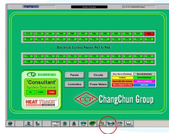
The front screen shows a representation of the areas managed by the Consultant system. The colour of each unit shown on this screen indicates its current operating state, flashing red indicates any units that have unaccepted alarms. Minor alarms (shown in orange) are primarily of interest to engineers only. These will not cause the alarm sounder to activate.
