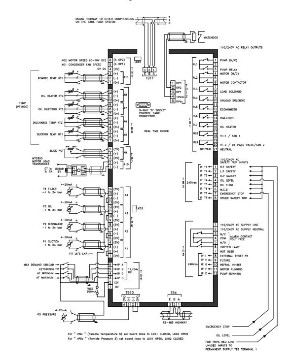
N.B. The Compressor Run Signal (TB3 Terminal 11) must be supplied to the Controller from the <u>Delta</u> Contactor of a Star-Delta System, or the <u>Top of Ramp</u> of a Soft Start System.
