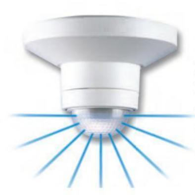
The PIR 360-F is equipped with three highly sensitive infrared detectors positioned at a specific angle in relation to each other to provide reliable, uninterrupted all-round protection of areas as large as 350 m² beneath it.
