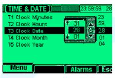
Use vertical arrows to select parameter setting to be changed and press **Enter**. This displays the setting change icon with setting value, maximum and minimum limits.
