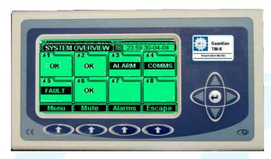
This Liquid Crystal Display (LCD) panel provides the local operator interface for up to **eight** Guardian GC1719 plant controllers.
