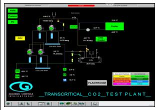
We have recently completed laboratory trials with the system running transcritically at 112barg via a heat exchanger to a dry cooler giving a gas cooler temperature o 44°C
