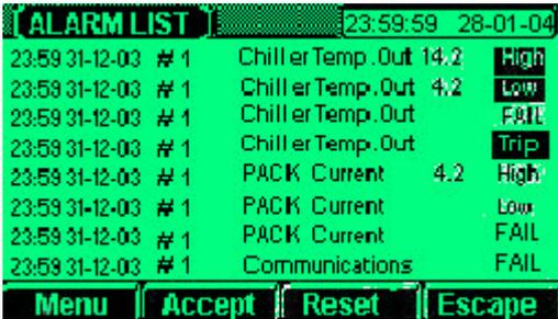
The **Alarm List** is displayed with most recent alarms at the top with eight messages per page. The alarm list holds the last 100 alarm messages generated for the system. Each message includes the time and date of occurrence, the system reference number and the reason for the alarm.
