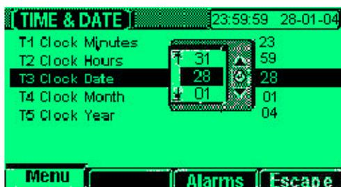
Use vertical arrows to select parameter setting to be changed and press **Enter**. This displays the setting change icon with setting value, maximum and minimum limits.
