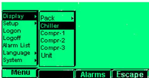
Further details of a particular section of the chiller are selected by using the keypad vertical and horizontal arrows to highlight the appropriate display tile name e.g. Chiller, Compressor 1 to 3 etc, followed by pressing **Enter**.
