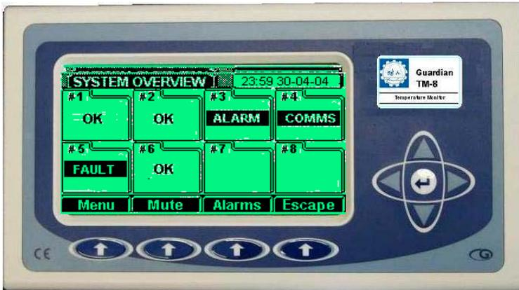
This Liquid Crystal Display (LCD) panel provides the local operator interface for up to **eight** Guardian GC1719 plant controllers.
