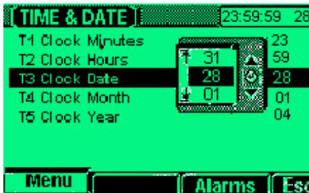
Use vertical arrows to select parameter setting to be changed and press **Enter**. This displays the setting change icon with setting value, maximum and minimum limits.
