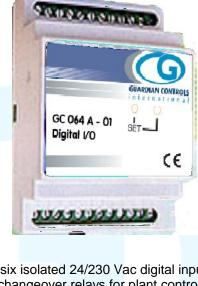
Provides six isolated 24/230 Vac digital inputs and four changeover relays for plant control. It may be used as a local Input/output extension to a plant or compressor controller or remotely as a mains input trip monitor or controller for a SCADA system.
