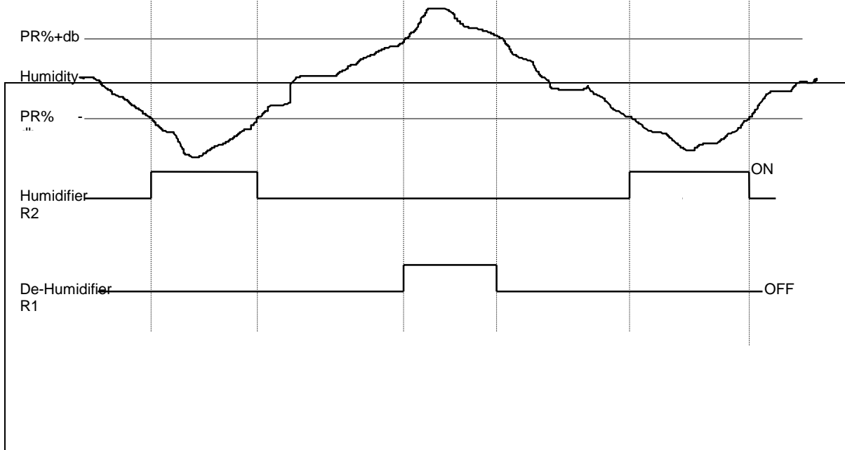
FIG.6 'HUNC' HUMIDIFIER & DE-HUMIDIFIER CONTROL
